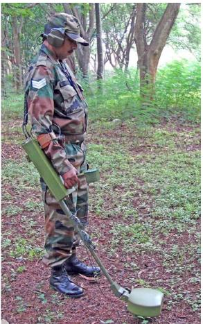
Figure 2: Indigenously realized Handheld GPR
