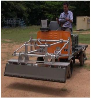
Figure 3: Indigenously Realized Vehicle Mounted GPR
