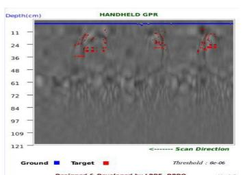
Figure 5: Detection of ATM buried at 9cm and swept over 3 times
