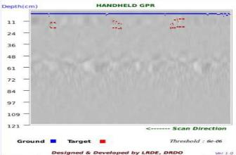
Figure 6: Detection of IED buried at 9cm and swept over 3 times
