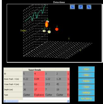
Figure 7: Detection of Influence Mine buried at 18 cm
